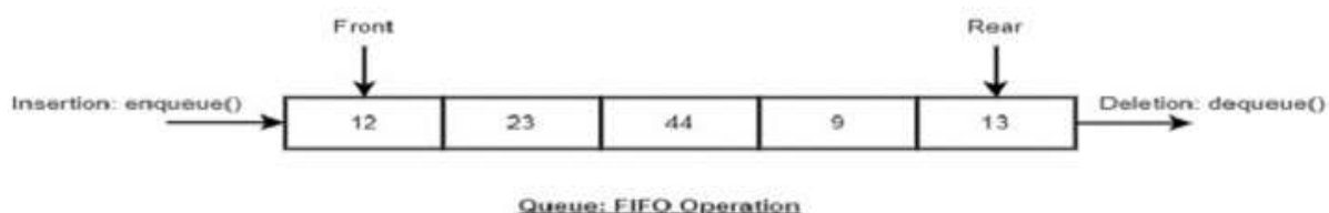
Fig. 5: Queue DS and its implementation in C
