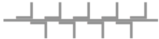
Fig. 8: Narrow-band bandstop filter design with nine resonators
