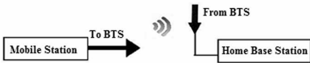
Figure 1: Point to point communication consisting of single base station and mobile station.
