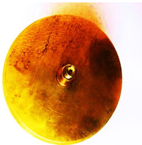
Fig.22. Prototype of Fabricated proposed continuous transverse stub antenna array (Front view).
