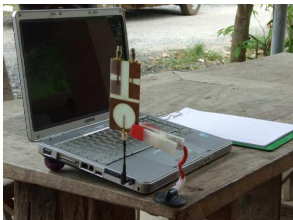
Fig. 12 Measurement setup under existing 3G scenarios.
