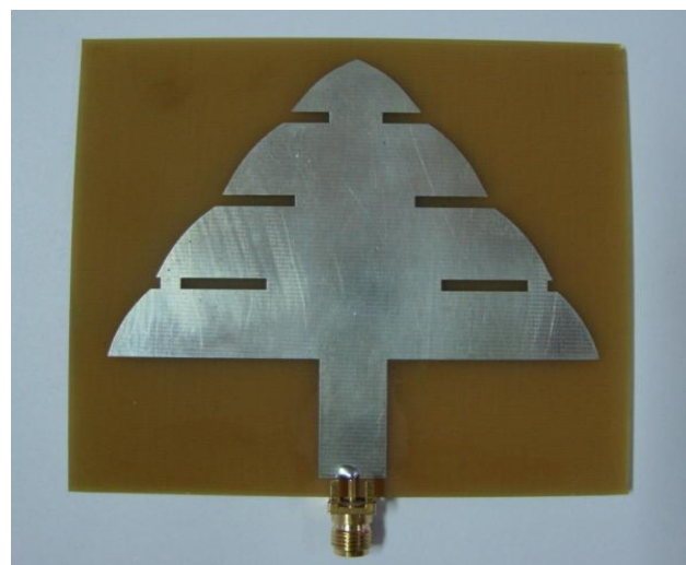
Fig.14. Fabricated microstrip patch antenna for CASE 1
