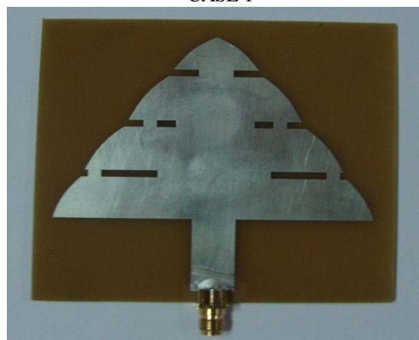
Fig.15. Fabricated microstrip patch antenna for CASE 2
