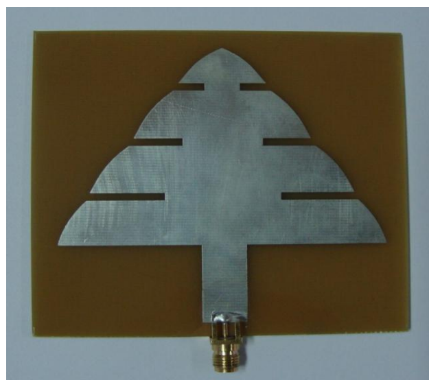
Fig.13. Fabricated microstrip patch antenna for CASE 0
