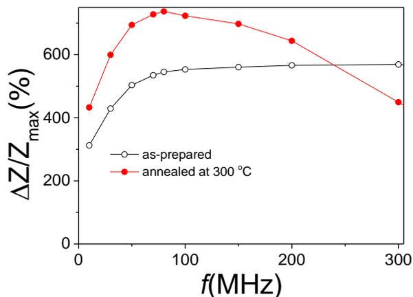
Fig.5.  $\Delta Z/Z_{\max}(f)$  dependences evaluated for as-prepared and annealed at 300 °C  $\text{Co}_{72}\text{Fe}_4\text{B}_{13}\text{Si}_{11}$  microwires.
