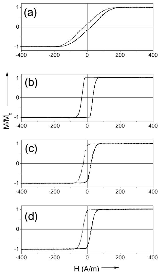
Fig. 3. Hysteresis loops of as-prepared (a) and annealed at  $T_{ann} = 275 \text{ }^\circ\text{C}$  (b),  $T_{ann} = 300 \text{ }^\circ\text{C}$  (c) and  $T_{ann} = 350 \text{ }^\circ\text{C}$  (d)  $\text{Co}_{72}\text{Fe}_4\text{B}_{13}\text{Si}_{11}$  sample.
