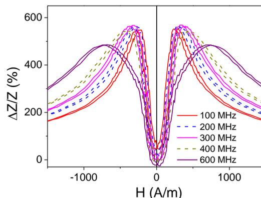
Fig.2.  $\Delta Z/Z(H)$  dependencies measured at different frequencies in studied as- prepared sample.
