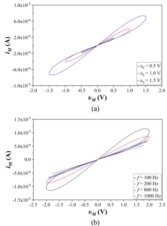
Fig. 1: Pinched hysteresis loops of the memristor model of Eq. (1), driven by different sinusoidal voltage stimuli  $v_M = V_m \sin(2\pi ft)$ , by using (a)  $f = 100$  Hz, with different values of voltage amplitudes  $V_m$ , and (b)  $V_m = 2$  V, with different values of frequencies  $f$
