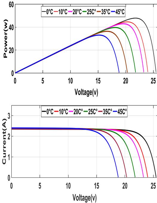
Fig. 3: Characteristics at different temperatures and irradiance levels
