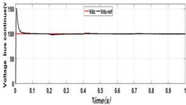
Fig. 12: DC bus voltage ( $V_{DC}$  and  $V_{DC-REF}$ ) due to irradiance changes in the conventional system
