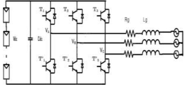
Fig. 5: DC-AC inverter model
