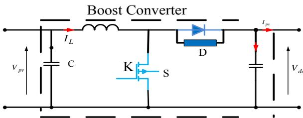
Fig. 4: DC/DC boost converter
