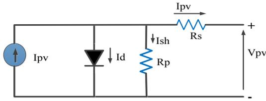
Fig. 2: Electrical model of the photovoltaic cell
