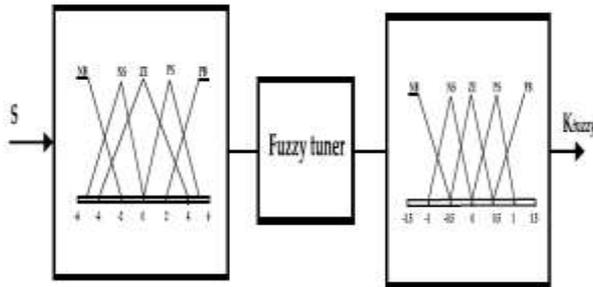
Fig. 8: Structural design of a tuner with fuzzy gain
