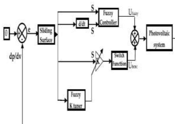
Fig. 7: Structure of the fuzzy-sliding mode control system
