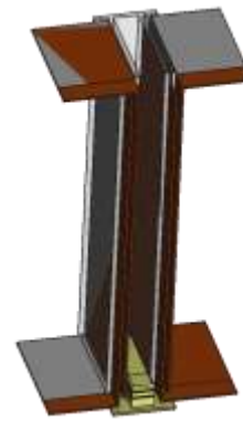
Fig. 1: A sectional cut of an orthogonal-shaped chamber using two pairs of electrodes
