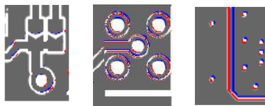
Fig. 13: Three examples of a difference between PCB fragments
