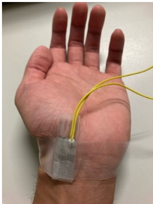
Fig02: Piezoelectric element taped to the wrist
