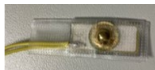
Fig09: Piezoelectric element with protrusion fixed with insulation tape
