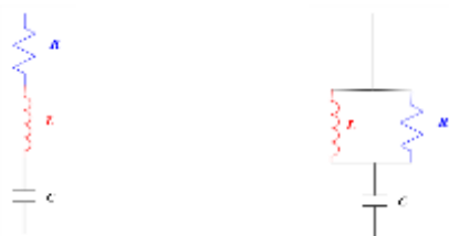
a) Resonant passive filter b) Damped passive filter Fig. 6: Types of Passive Filter
