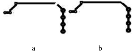
Fig. 17. Open defect (a) and correct chain (b)
