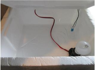
Fig. 3 Internal layout of a closed space in a constant humidity control experiment. There are DHT11 temperature/humidity sensor and a 40(W) incandescent light bulb.
