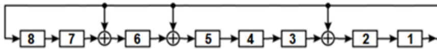
Fig. 15. Block diagram of the "reverse" generator PRN in the Galois configuration generated by the PrP f_8 = 101100101
