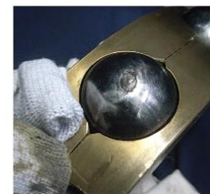
(a) Rolling element wear
