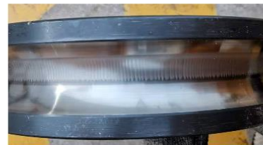
(b) Inner ring failure
