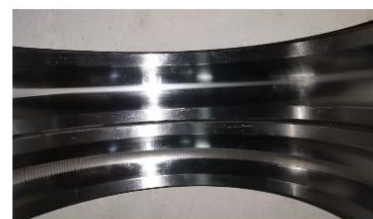
(c) Outer ring fault
