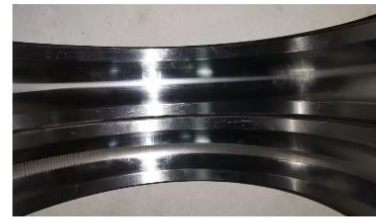
(c) Outer ring fault
