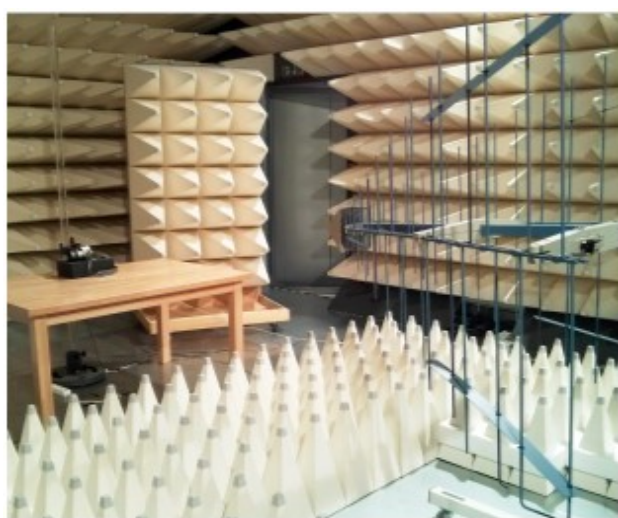
Fig. 7 Configuration of the experiment inside the semi anechoic chamber; part of the transmitting antenna can be seen on the right side while the tested camera is put on the wooden table in the distance of 3 meters
