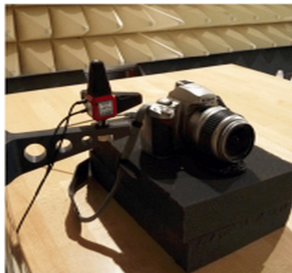
Fig. 8 Configuration of the experiment inside the semi anechoic chamber; camera put on the wooden table with a feedback probe behind
