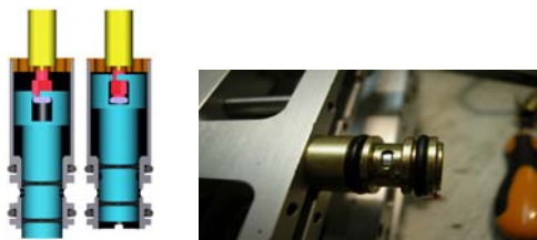
Fig. 5. The picking module in open and closed positions and a physical prototype
