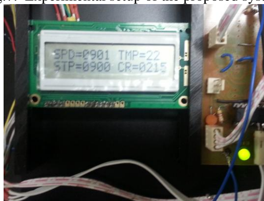
Fig.8. The motor parameters read by the system after the command speed is executed.
