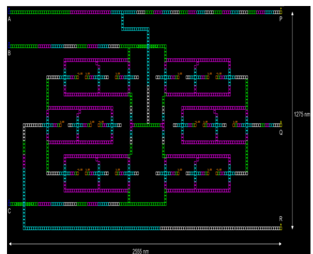
Fig. 15. QCA implementation of FREDKIN gate
