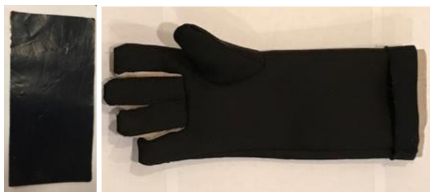
Fig.2: Example application: CNT fabric used as a center layer in a prototype glove for firefighting.
