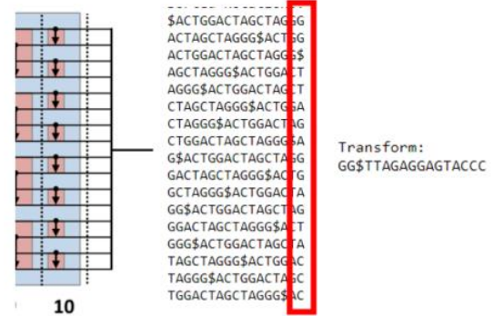
Fig. 5: The concatenation of the last 4-bits to obtain the Last Column of the BWT transform process
