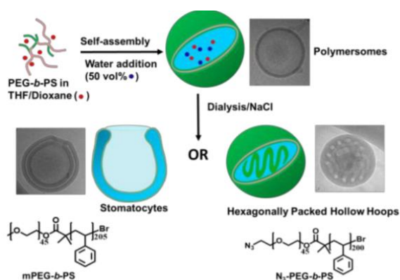
Fig. 12: Schematics of shape transformation of polymersomes either into stomatocytes or HHHs. Adapted from [29]
