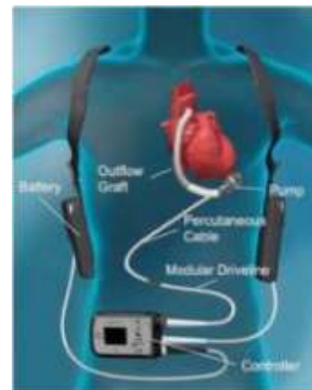
Fig. 1: VAD with batteries, controller, and peripheral systems. Adapted from, [5]
