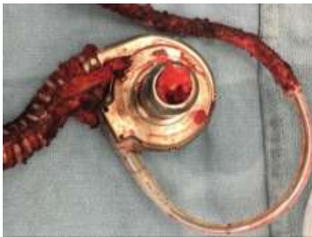
Fig. 2: Thrombus formation in a removed VAD. Adapted from, [9]
