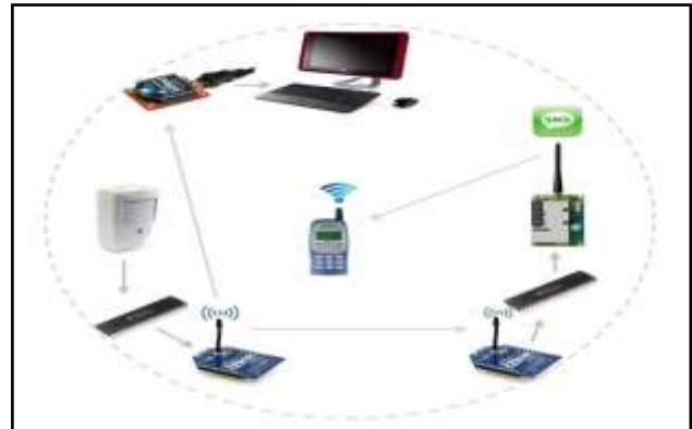
Figure 1.1 Wireless alarming systems Diagram
