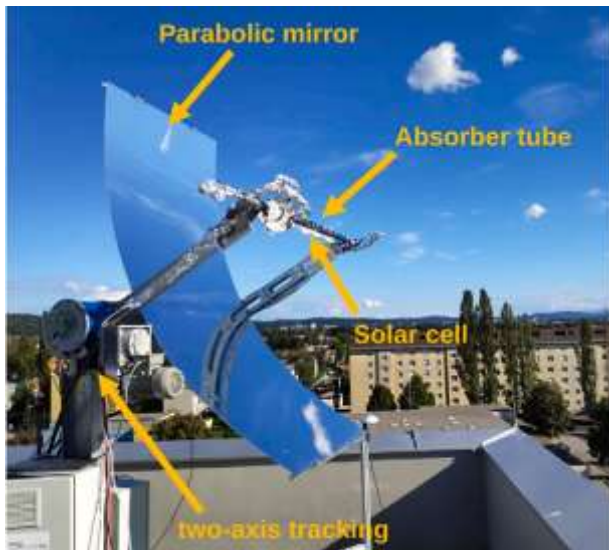
Figure 14. A parabolic trough with solar cells [33].
