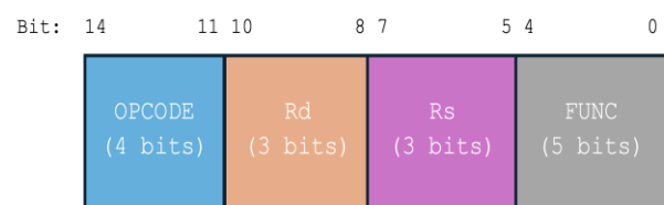
Fig. 2: AURORA-15 Format-A instruction bit-field structure for arithmetic and logical operations
