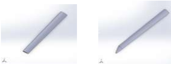
Figure 2.a) Conventional wing Figure b) Raked winglet 25° [12].
