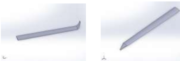
Figure 3 a) Blended winglet 30° b) Raked winglet with chevron.
