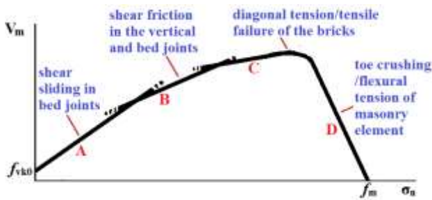
Fig. 19: Failure envelope for masonry element, [15], [13], expressed in terms of shear strength ( V_m ) versus compressive stress ( \sigma_n ), with four main failure modes, A to D ( f_{vk0} - initial shear strength of masonry; f_m - compressive strength of the masonry)
