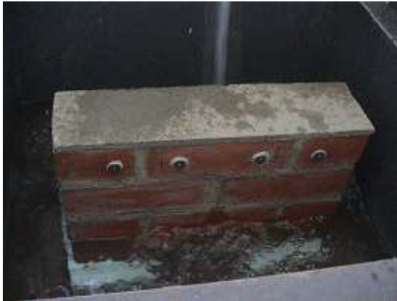
Fig. 3: The phase of immersion in water during 24 hours of the Specimen M1
