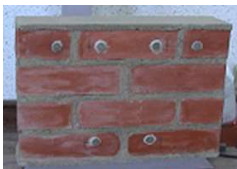
Fig. 4: The phase of preparation of the Specimen M1 for the 1 st phase of the compression test
