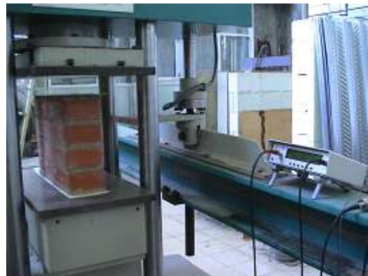
Fig. 6: Aspect of face A of Specimen M1 before the compression test
