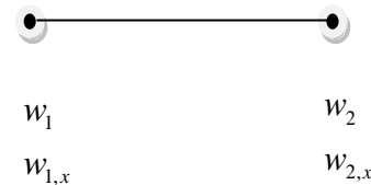
Fig. 2: Finite beam element.
