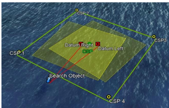
Fig. 14 – Iamsar model simulation for person in water under unknown conditions with d = 0.62, E = 1.44\text{NM}, \text{POS} = 77.2\%, f_s = 1.46 e C = 1.37 - Square area – Weather condition with sea force 2 and discrete visibility
