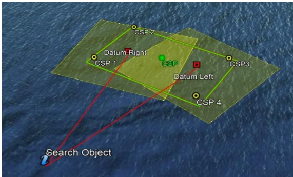
Fig. 13 – Advanced model simulation for 5 mt sport fishing boat, with d = 1.56, E = 6.67\text{NM}, \text{POS} = 36.9\%, f_s = 0.90 e C = 0.77 – Rectangle area – Weather condition with sea force 2 and discrete visibility
