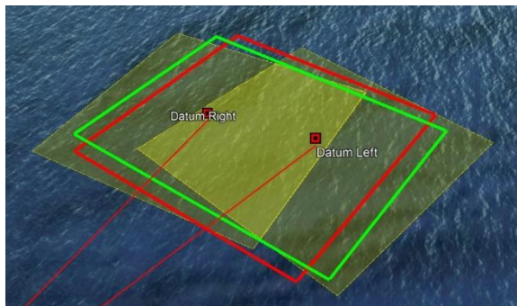
Fig. 3 - Comparison between areas with unitary search factor f_s=1 of the single punctual datum POC (square) and the divergent datum POC (rectangle) with d=1.15 and E=4.66 NM
