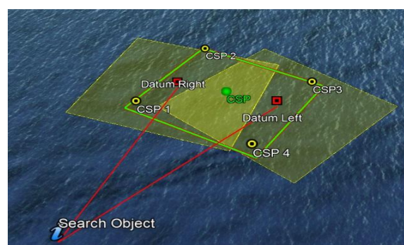
Fig. 12 – Iamsar model simulation for 5 mt sport fishing boat, with d = 1.56, E = 6.67\text{NM} , POS = 33.5\% , f_s = 0.87 e C = 0.82 – Square area – Weather condition with sea force 2 and discrete visibility
