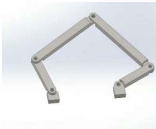
Fig.2 5R robot modelled by Solid Works Software
