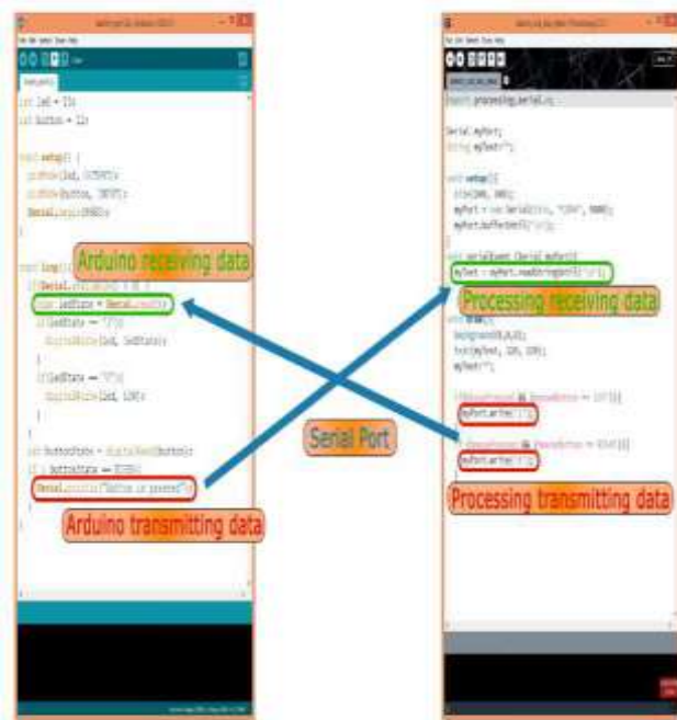
Fig. 8. Arduino and processing software connection image
