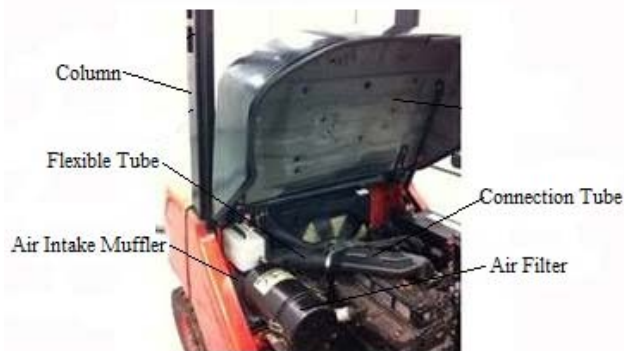
Fig. 1 the components of IC forklift intake system
