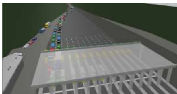
Fig. 5: Formation of congestion on manual toll lanes of a reversible TP. General view
