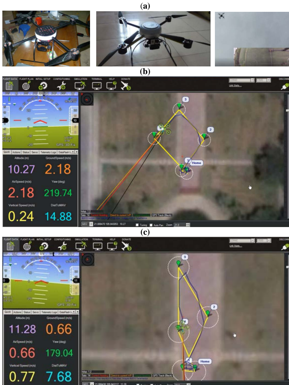
Fig. 10. Setting up and testing the controller for the developed autonomous quadrotor UAV (a); Quadrotor UAV reaches and follows a desired rectangle-shaped trajectory with steer angles about 90^\circ (b); Quadrotor UAV reaches and follows a desired quadrangular-shaped trajectory with steer angles about 120^\circ , 30^\circ and 150^\circ (c).
