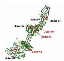
Fig.2. The 7-joints Robot Arm.
