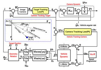
Fig.5. Tracking and Control Configuration of Horizontal Plane.
