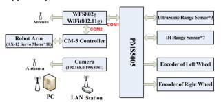
Fig.3. System Hardware Interface.
