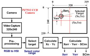
Fig.8. Data Processing Flow Chart & Parameter Definition.
