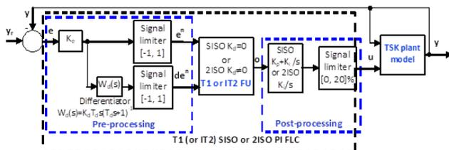
Fig. 1: Closed loop system with T1 PI FLC on SISO or 2ISO FU for control of TSK plant model
