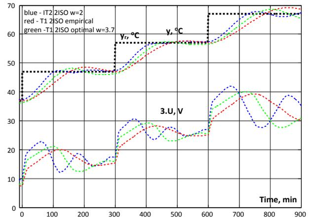
Fig. 8: Step responses with respect to temperature and control action of T1 and IT2 2ISO PI FLC systems
