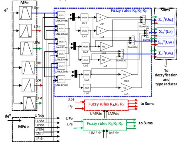
Fig. 5: Simulation model of IT2 2ISO FU
