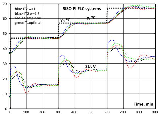
Fig. 7: Step responses with respect to temperature and control action of T1 and IT2 SISO PI FLC systems
