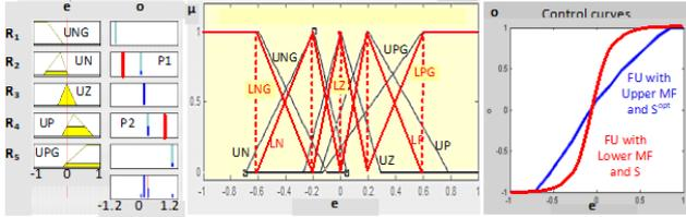
Fig. 4: Fuzzy rules, MF, singletons, and control curves of empirically designed T1 FU ( $MFe=LMF, S$ ) and GA optimised T1 FU<sup>opt</sup> ( $UMF, S^{opt}$ )
