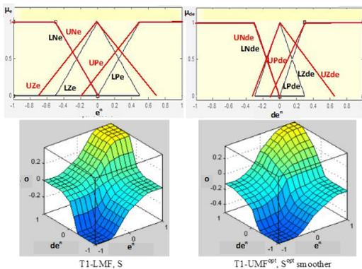
Fig. 6: LMF and UMF and control surfaces for T1 FU with (LMF, S) and T1 FU<sup>opt</sup> with (UMF<sup>opt</sup>, S<sup>opt</sup>)
