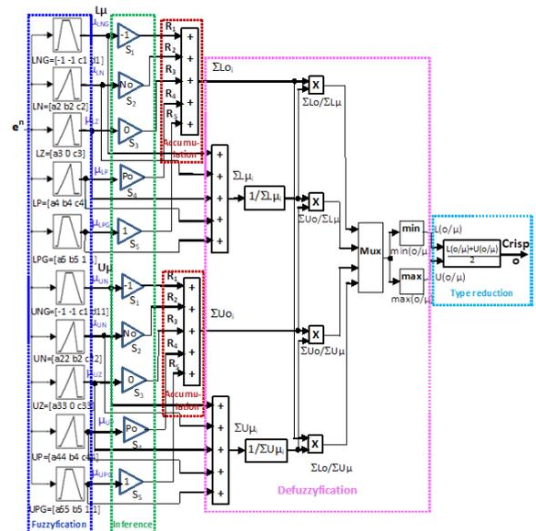
Fig. 3: Simulation model of IT2 SISO FU
