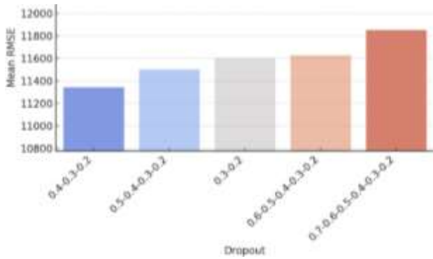
Fig. 11: Average RMSE for different dropout patterns
