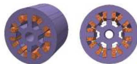
Fig. 1: 3D projection of 8/6 SRM obtained by FEM analysis.
