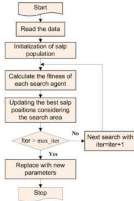
Fig. 5: SSA utilized for the best balance of voltage and current flow chart, [19]
