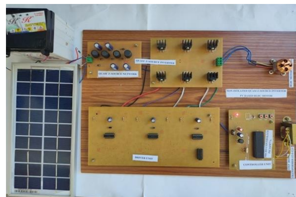
Fig. 12: Hardware prototype of Proposed QZSI
