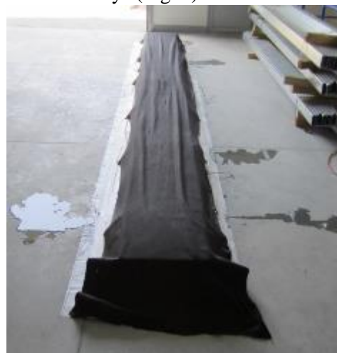
Fig. 3 Laboratory specimen covered with wet geotextile
