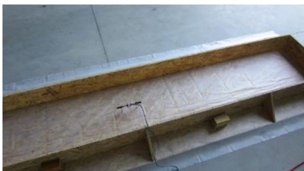
Fig. 2 Formwork with PE foil and installation of internal string strain gauges
