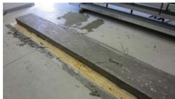
Fig. 4 Large-dimensional sample in the laboratory and installation of external string strain gauge
