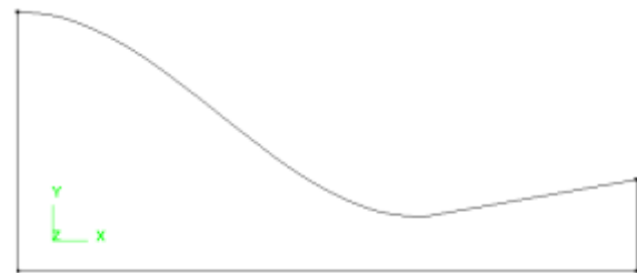
Fig. 1: The nozzle profiles employed in the 2D calculations
