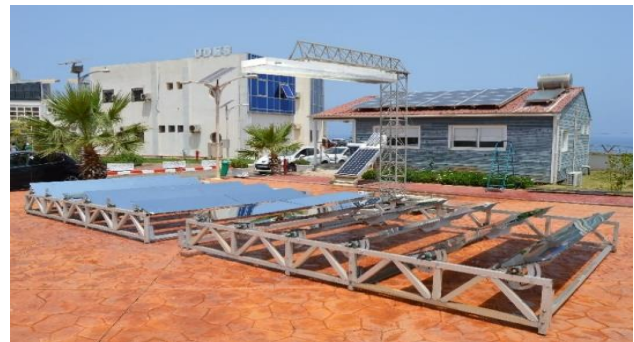
Fig. 1. LFC prototype for experimentation realized at UDES [10-12]
