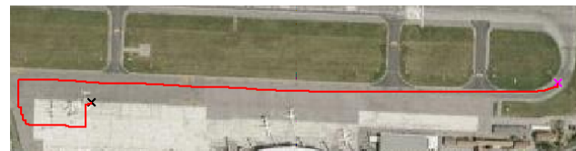
Figure 17: Modified HNN. Arrival Mission: Phase 2, from aircraft landing waiting position to parking lot. Credits: Pictures 2015 DigitalGlobe, Map data ©2015 Google.
