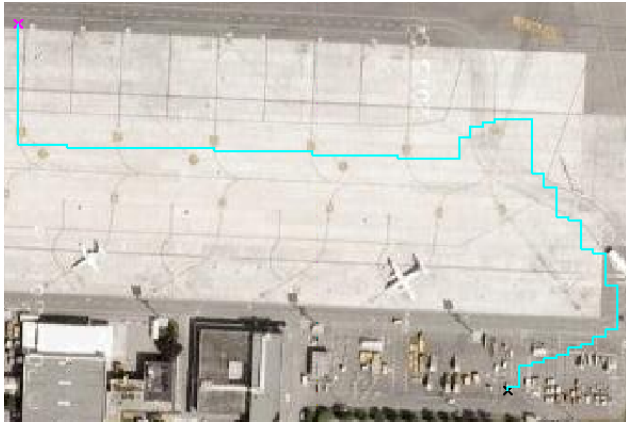
Figure 18: Modified HNN. Arrival Mission: Phase 3, from aircraft selected parking lot to tractor deposit. Credits: Pictures 2015 DigitalGlobe, Map data ©2015 Google.1
