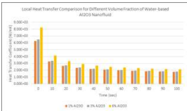
Fig. 10: Local Heat Transfer Comparison for Different Concentrations of Al 2 O 3 -water nf
