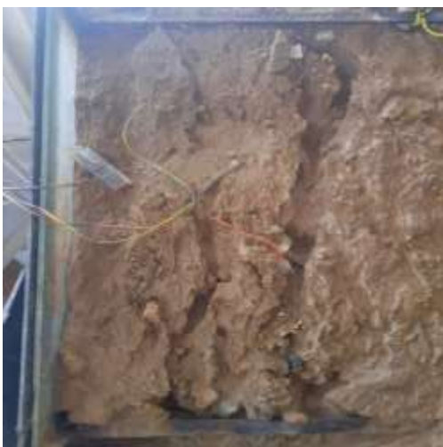
Figure 4 Experimental set up when soil moisture value goes to 90 percent of the maximum value
