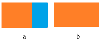
Fig. 4: Two flood-filled images: red pixel as starting point (a) and blue pixel as starting point (b)
